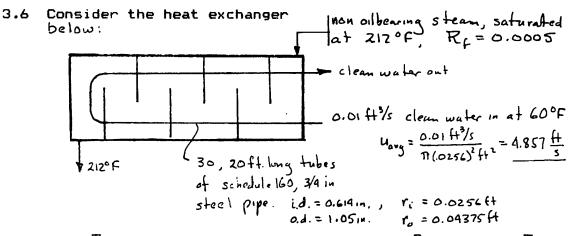
Take  $\overline{h}$  inside the tubes to be 1380 Btu/ft<sup>2</sup>-hr-<sup>O</sup>F and  $\overline{h}_{cond}$  as 2000 Btu/ft<sup>2</sup>-hr-<sup>O</sup>F.
