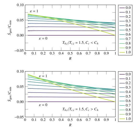
Another way to approach this is to plot  $\dot{S}_{gen}/C_{min}$  for fixed  $T_{h,i}/T_{c,i}$  and several values of  $\varepsilon$ .
