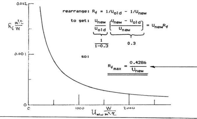
3.19 Plot R<sub>f</sub> <u>vs.</u> U<sub>new</sub> if a 30 % reduction in U is the maximum tolerable.
