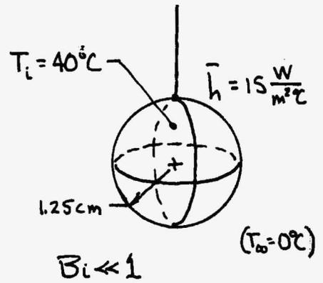
$$\text{so: } \tau = \frac{\rho c D}{6\bar{h}} = \frac{\text{m}^2\text{C}}{\text{C}(\text{W})} \cdot \frac{8954 \text{ kg}}{\text{m}^3} \cdot \frac{384 \text{ J}}{\text{kg}^\circ\text{C}} \cdot (0.025 \text{ m}) \cdot \left(\frac{\text{W}\cdot\text{s}}{\text{J}}\right) = \frac{955 \text{ sec}}{= 15.92 \text{ min.}}$$
