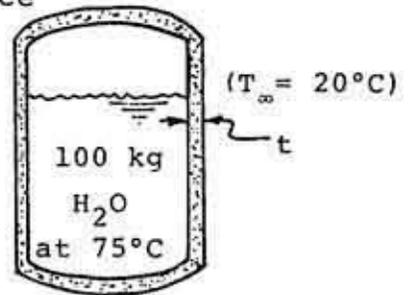
First determine the heat flux:  $q = \frac{Q}{A} = \frac{(\text{mass})c}{A} \frac{dT}{dt} = \frac{(100)(4190)3}{1.3(3600)}$
