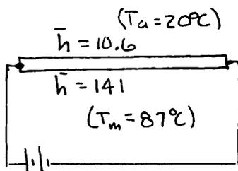
$$q_{\text{to plate from meth.}} + q_{\text{elect. to plate}} = q_{\text{to air from plate}}$$
