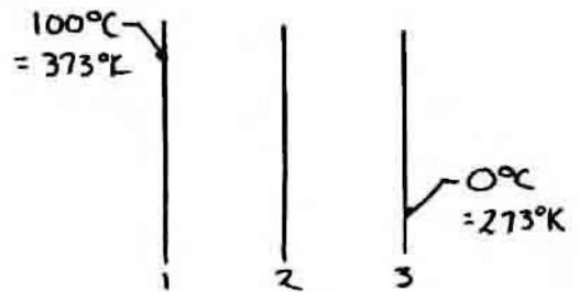
$$q = \sigma(T_1^4 - T_2^4) = \sigma(T_2^4 - T_3^4) \quad \text{so} \quad 2T_2^4 = T_1^4 + T_3^4$$
