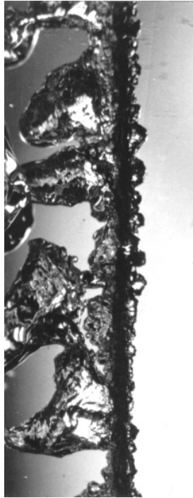
3.75 cm length of 1.64 mm diam. wire in benzene at earth-normal gravity. q = 0.35 \times 10^6 \text{ W/m}^2
